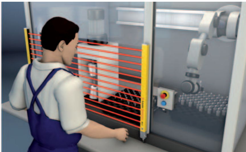
MLC 300 Safety Light Curtain guarding an assembly cell with manual access
