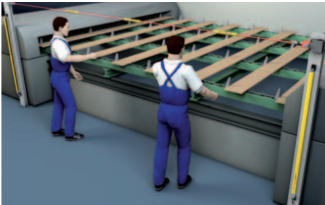
The ERS200 E-Stop Rope Switch is used as a Safety Command Device in expansive hazard locations
