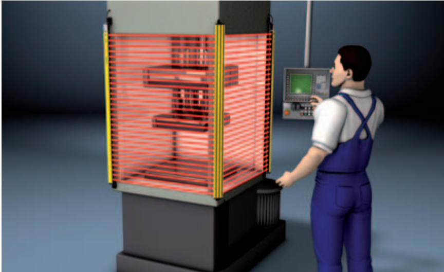
MLC 500 Safety Light Curtain for hand and finger protection
