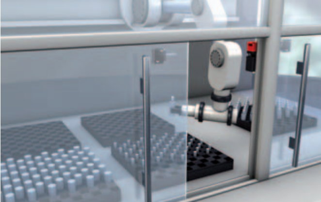
Safety Switch for guarding the sliding door on a pick-and-place machine
