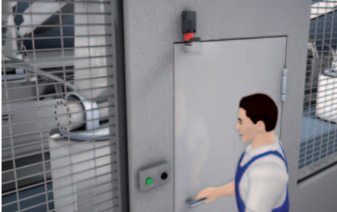
Safety Locking Device as access guarding
