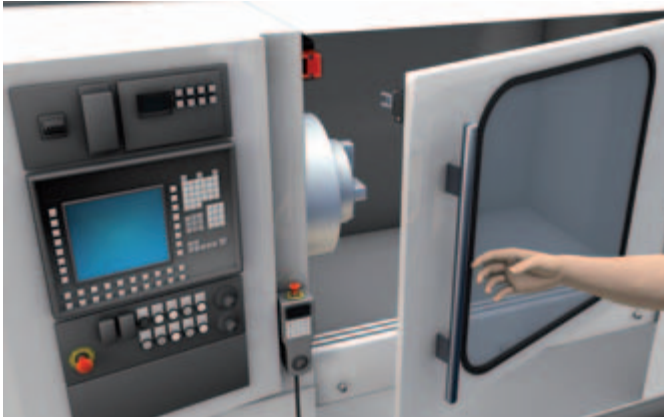
Safety Locking Device on a metal processing center with stopping times
