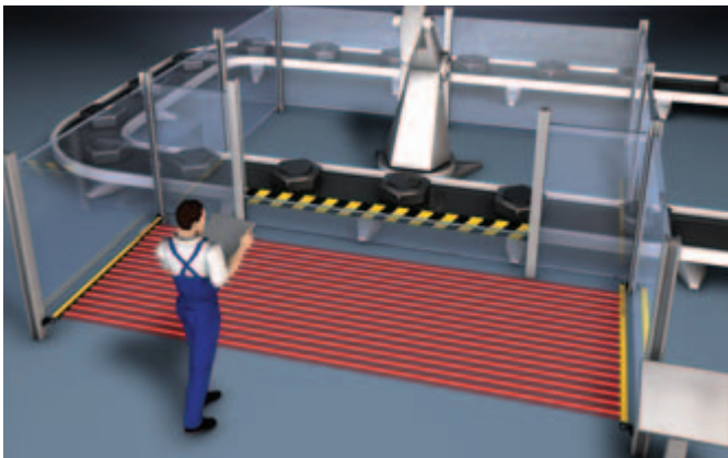
Safety Light Curtain with an MSI-SR4 Safety Relay as danger zone guarding with start/restart interlock on a robot cell
