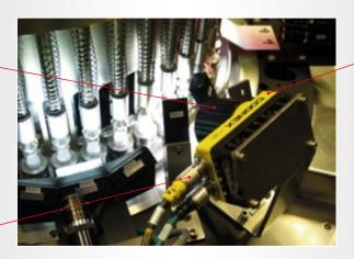
Standard Housing Die-cast and steel cases are IP67 (NEMA 6) rated and have a protective lens cover.
