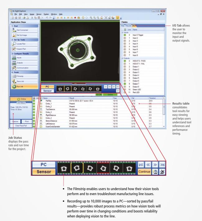
• Recording images directly to the vision system allows operators and technicians to understand why parts are passing or failing in real time, without halting the vision system.
