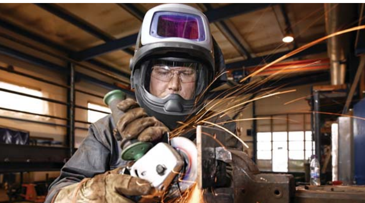
A spark- and spatter-resistant fabric head cover is standard on all Speedglas 9100 FX Series Welding Shields.
