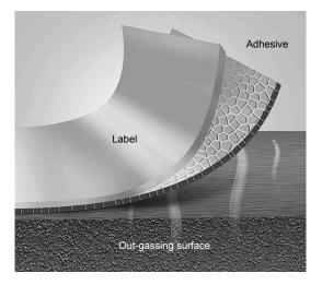
These label materials are designed for use at Narrow Web & Screen Print Converters and OEM's who need to apply bubblefree product identification decals and graphics for long-term durability. 3M<sup>™</sup> Performance Labels with Structured Adhesive can be applied wrinkle and bubble-free, even on plastics that are prone to out-gassing, reducing costly rework & scrap.
