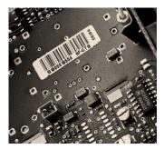
A high temperature-resistant label is applied to the face of a PCB to allow tracking around the manufacturing plant during board population, flow solder and drying processes. ■ 3M<sup>TM</sup> Cast Acrylic High Temperature Label Materials are thermal transfer printable,
