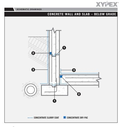
Step 2 In sealing strip, apply one slurry coat of Xypex Concentrate at the rate of 1.5 lb./sq. yd. (0.8 kg/m<sup>2</sup>) then fill slot to surface with Xypex Concentrate in Dry-Pac form.
