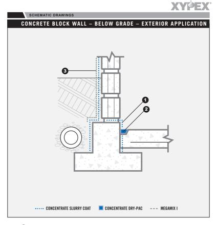
Step 1 Prior to placement of the concrete wall and slab, apply one slurry coat of Xypex Concentrate to joint surfaces at the rate of 2 lb./sq. yd. (1 kg/m<sup>2</sup>).
