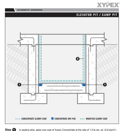
In sealing strip, apply one coat of Xypex Concentrate at the rate of 1.5 lb./sq. yd. (0.8 kg/m<sup>2</sup>), then fill slot to surface with Xypex Concentrate in Dry-Pac form.
