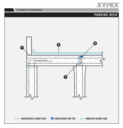
Step 2 In sealing strip, apply one coat of Xypex Concentrate at the rate of 1.5 lb./sq. yd. (0.8 kg/m<sup>2</sup>), then fill slot to surface with Xypex Concentrate in Dry-Pac form.
