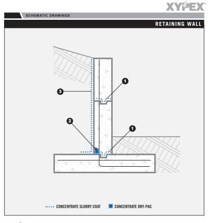
In sealing strip, apply one slurry coat of Xypex Concentrate at the rate of 1.5 lb./sq. yd. (0.8 kg/m<sup>2</sup>), then fill slot to surface with Xypex Concentrate in Dry-Pac form.
