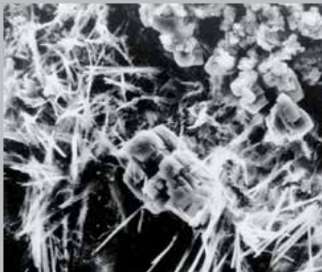
XYPEX CRYSTALLIZATION (INITIATION)
