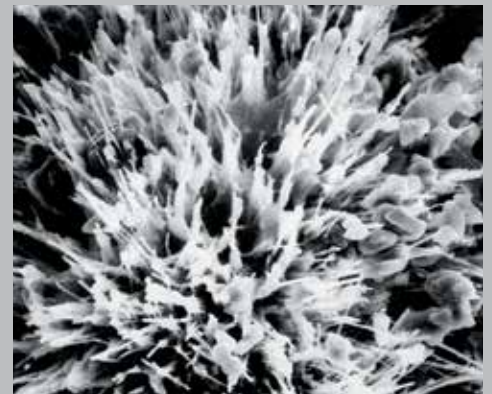
XYPEX CRYSTALLIZATION (MATURE)
