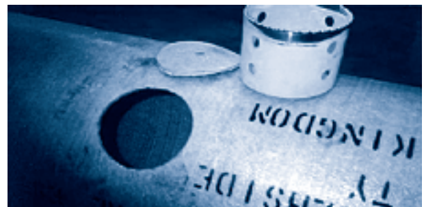
Figure 8-4 Alternative cutter with closely spaced teeth
