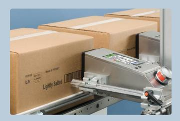
The Videojet<sup>®</sup> 2300 series is a family of three high resolution, large character ink jet printers that provide class-leading, consistent print quality on porous and secondary packaging materials. These systems are designed and manufactured to reliably print accurate, high quality, real time alphanumeric codes, bar codes and graphics with a range of printhead heights to best suit your printing needs.
