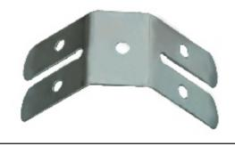
Spring steel with Delta protect treatment. Metal accessory to be used for the construction of suspended ceilings. The accessory is fitted by double threading to the various types of hanger.
