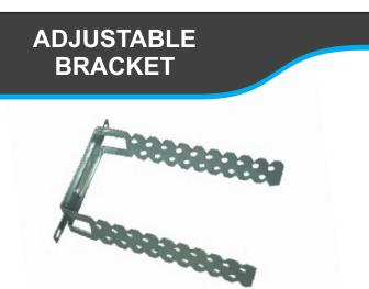
Galvanized steel, used for the construction of wall linings with 30 mm to 120 mm profile section-wall base spacing. Fitting is by means of bracket-profi le section coupling, at pre-established height by using structural screws, turning the ends towards the inside of the wall, the additional length of the bracket is re-positioned.
