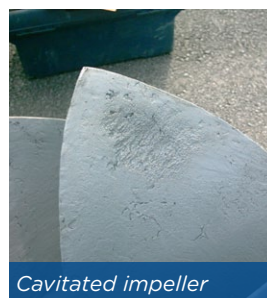
Erosion on internal surfaces of pump
