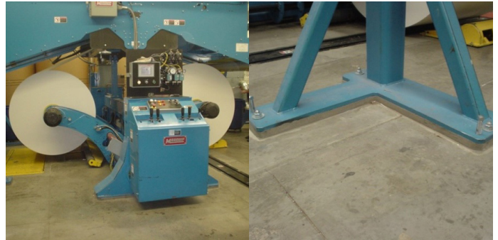
Hydraulic paper cutter installed
